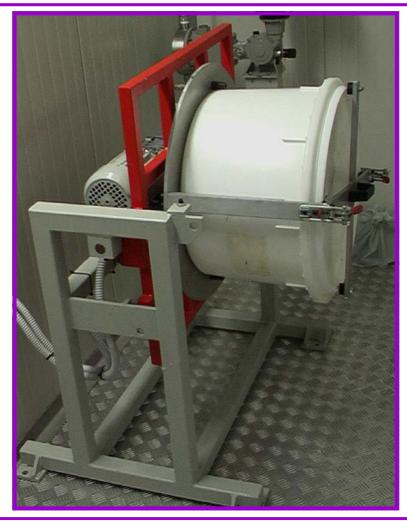
The mixer is an ancillary machine for mixing of P.T.F.E. powders with its Iso-paraffinic lubricant.
